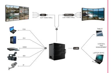
**Overview** The UltraVista Pro Video Wall processor accepts a wide variety of video input signals for display on screens grouped as video walls. The input signals can be processed and combined for the optimal viewer experience.
